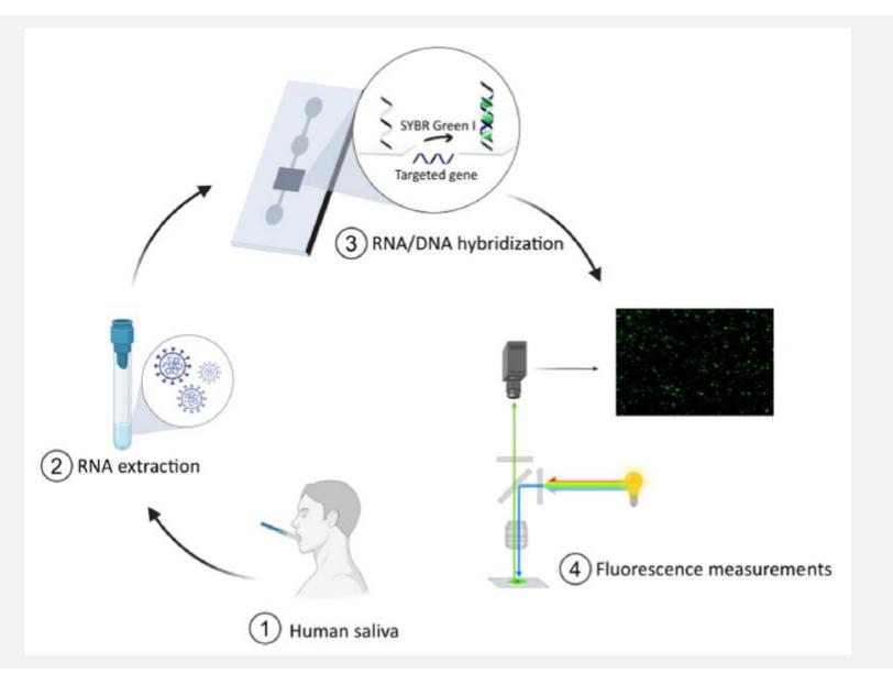
Specific probe was designed and covalently immobilized at the surface of glass slides to fabricate a DNA biosensor, allowing the identification of viral charge by the detection of RNA/DNA hybridization events at the surface of the sensing slides.
